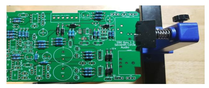
6. Add the small ceramic capacitors. These capacitors are not polarized and can be installed in either direction, but pay close attention to the capacitor markings! These parts all look alike, but they are not interchangeable. Putting one in the wrong spot will not prevent the preamp from passing signal, but it can seriously impair its performance.
