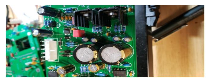
**14.** Add bulk electrolytic capacitors C2, and C6. Again, **electrolytic capacitors are polarized and must be installed the right way around!** Be absolutely sure to observe the correct polarity when installing these parts.
