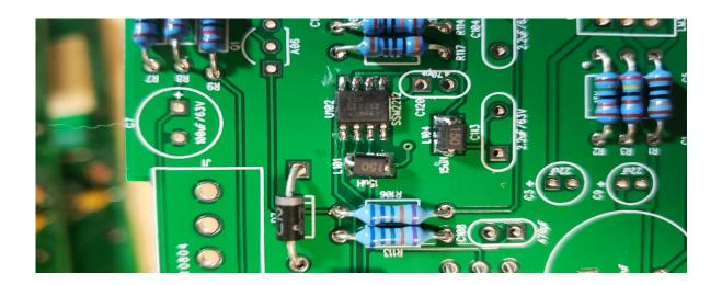
8. Install all other 8-pin IC's now. Pay close attention to the IC markings. Align the notch on the IC with the notch on the silkscreen outline! IC sockets are not included in the kit and are not recommended. Socketing the ICs will interfere with the ability of the PC board to conduct heat away from the parts.
