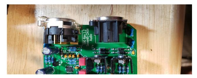
**18.** Before going on to initial power-up, carefully check your work. Make sure you haven't created any solder bridges between pads, or between a pad and the ground plane.
