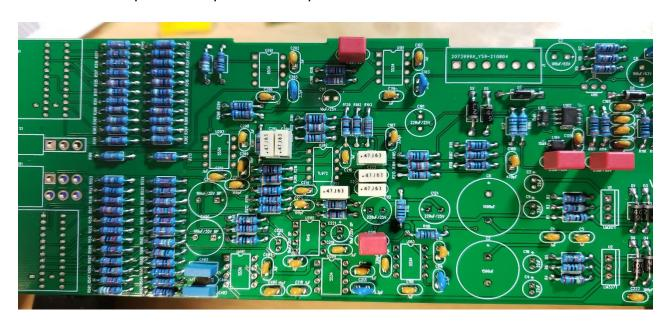
11. Add the shorter electrolytic capacitors now, followed by the taller. "BP" caps are not polarized, but the rest are **and must be installed the right way around!** Be absolutely sure to observe the correct polarity when installing these parts. The **negative leads** of the electrolytic caps are marked with a colored stripe. The **positive pads** on the circuit board are marked with a small "+" sign.
