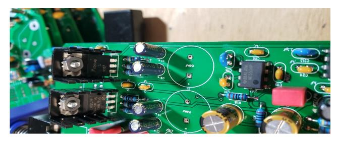
**16.** Install rotary switches. Make sure the switches are fully seated and solder them to the board. Try to make your solder joints as neat as possible, and don't use too much solder.
