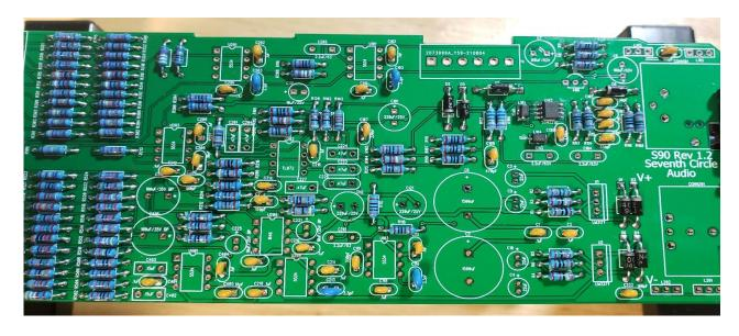
7.Install the SMT components U102, L101, and L104 now. Use plenty of flux! Pay close attention to the IC marking. Align the dot on the IC with the notch on the silkscreen outline
