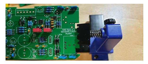
**10.** Install the film caps. These parts are not polarized and can be installed in either direction.
