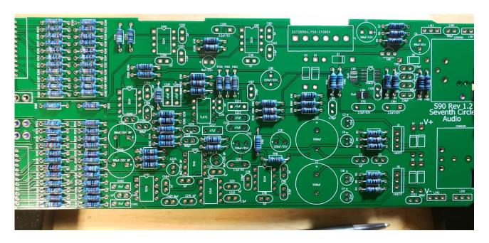
5. Next, add the protection diodes. Diodes are polarized and must be installed the right way around! The colored band on the diode matches the white band on the silkscreen.
