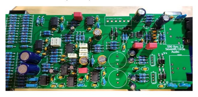
**9.** Install the blue EMI filters now. These parts are not polarized and can be installed in either direction.
