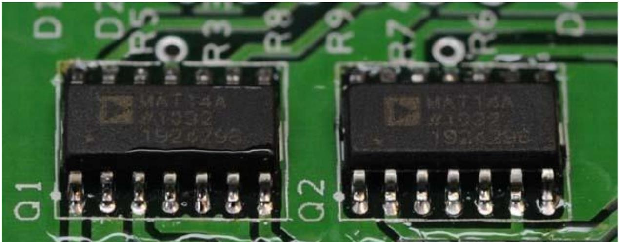
10. Install U1, U2, and U3 now. **Pay close attention to the IC markings. Align the notch on the IC with the notch on the silkscreen outline!** IC sockets are **not included** in the kit and are **not recommended**. Socketing the ICs will interfere with the ability of the PC board to conduct heat away from the parts.
