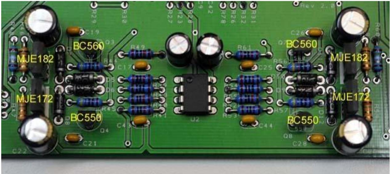
15. Add Q11 and Q12. Again, these parts are not the same, and are not interchangeable. **Align the flat side of the transistors with the flat side of the silkscreen outline.**
