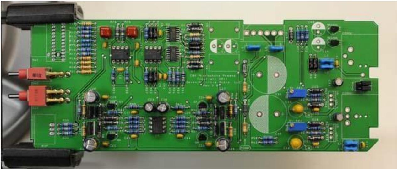
21. Add J3, the MOLEX power connector. Be sure to orient it as shown, with the locking tab away from the edge of the board.
