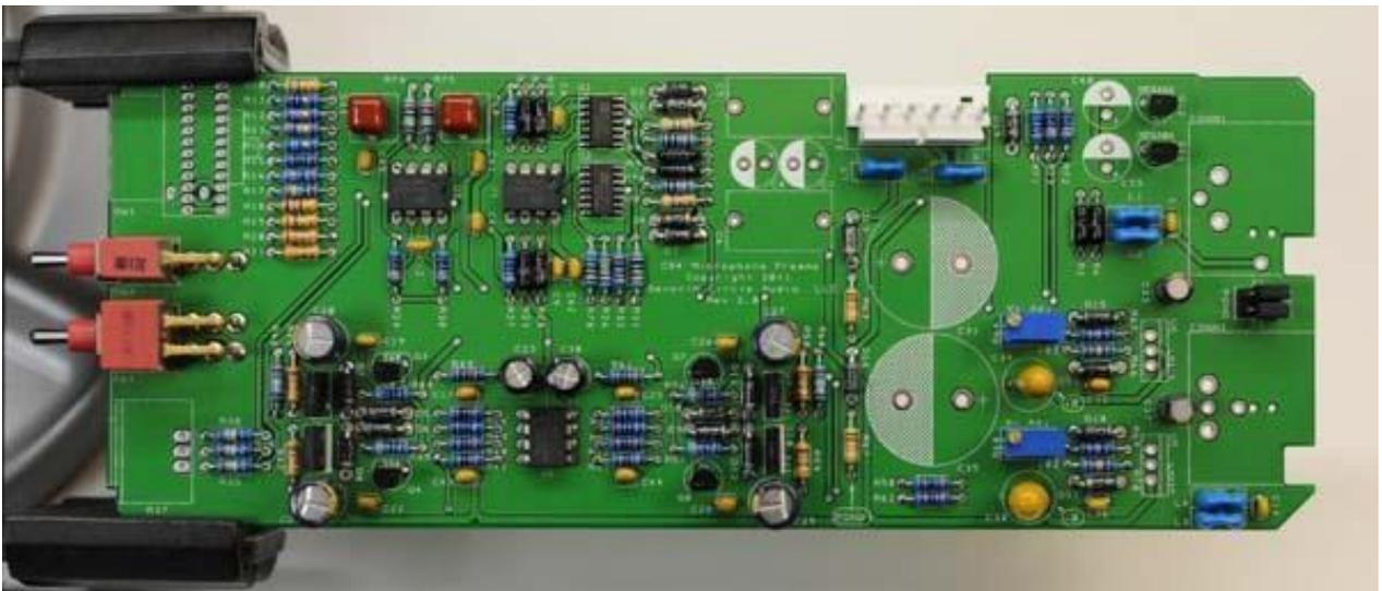
22. Add electrolytic capacitors C4, C7, C39 and C40. Again, **electrolytic capacitors are polarized and must be installed the right way around!** Be absolutely sure to observe the correct polarity when installing these parts. Add polypropylene capacitors C5 and C6 as well.
