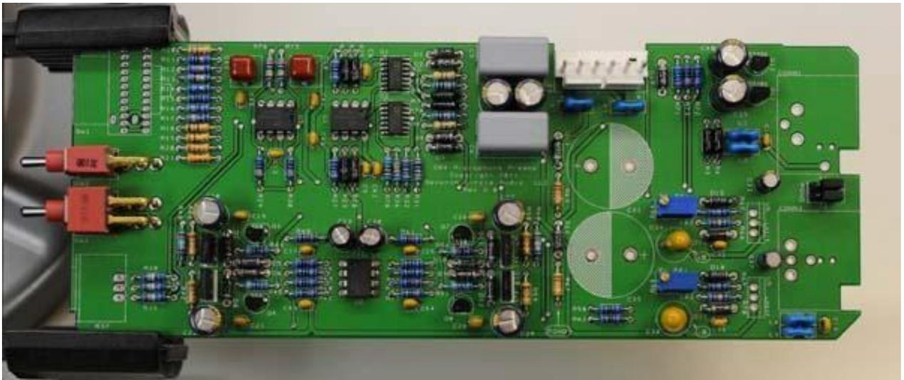
24. Using the hardware supplied, attach heat sinks to U5 and U6 and solder them in place. **Make sure to install the regulators correctly!** These parts are not the same and are not interchangeable.
