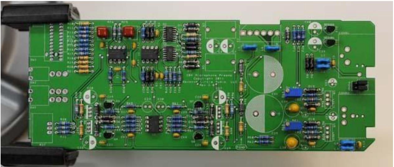
18. Add the short electrolytic capacitors now. C23 and C30 are not polarized, but the rest are **and must be installed the right way around!** Be absolutely sure to observe the correct polarity when installing these parts. The **negative leads** of the electrolytic caps are marked with a colored stripe. The **positive pads** on the circuit board are marked with a small "+" sign.
