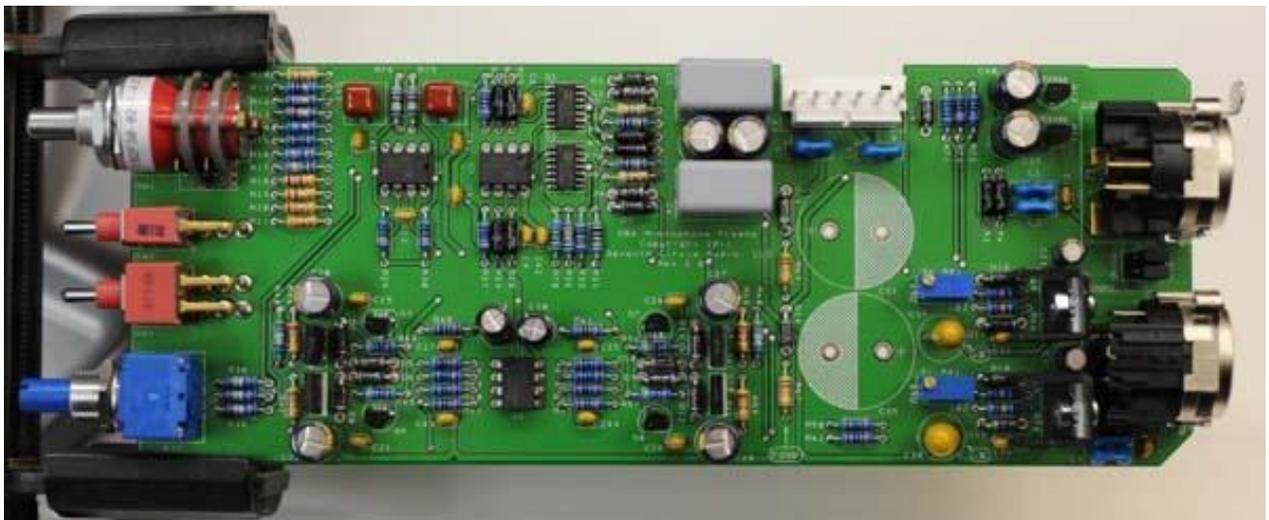
28. Install the bulk filter capacitors C31 and C35. Push them in firmly until they are fully seated against the board. Again, **electrolytic capacitors are polarized and must be installed the right way around!** Be absolutely sure to observe the correct polarity when installing these parts.
