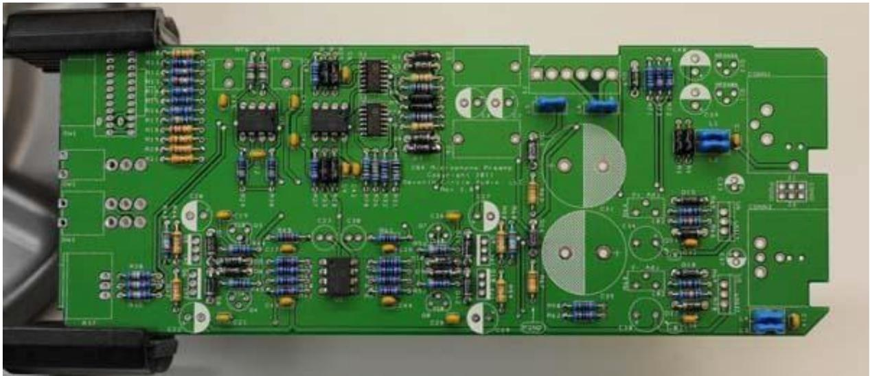
14. Add small transistors Q3, Q4, Q7, and Q8. These parts are not the same and are not interchangeable. **Align the flat side of the transistors with the flat side of the silkscreen outline.**
