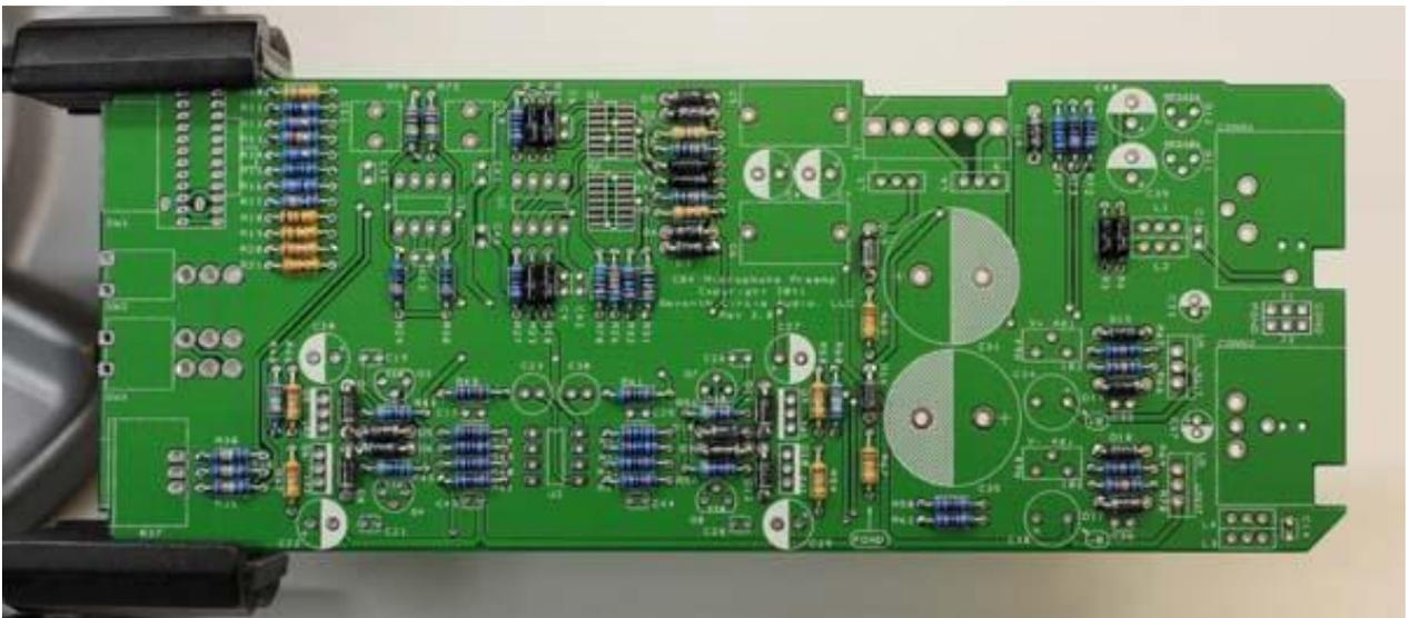
6. Add the small ceramic capacitors. These capacitors are not polarized and can be installed in either direction, **but pay close attention to the capacitor markings!** These parts all look alike, but they are not interchangeable. Putting one in the wrong spot will not prevent the preamp from passing signal, but it can seriously impair its performance.
