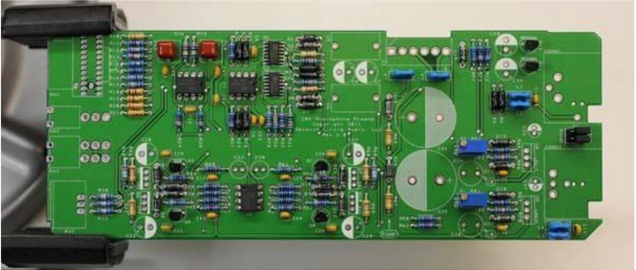
17. Add tantalum capacitors C34 and C38. **Tantalum electrolytic capacitors are polarized and must be installed the right way around!** Be absolutely sure to observe the correct polarity when installing these parts. The **positive leads** of the tantalum caps are marked with a small "+" sign. The **positive pads** on the circuit board are marked with a small "+" sign.
