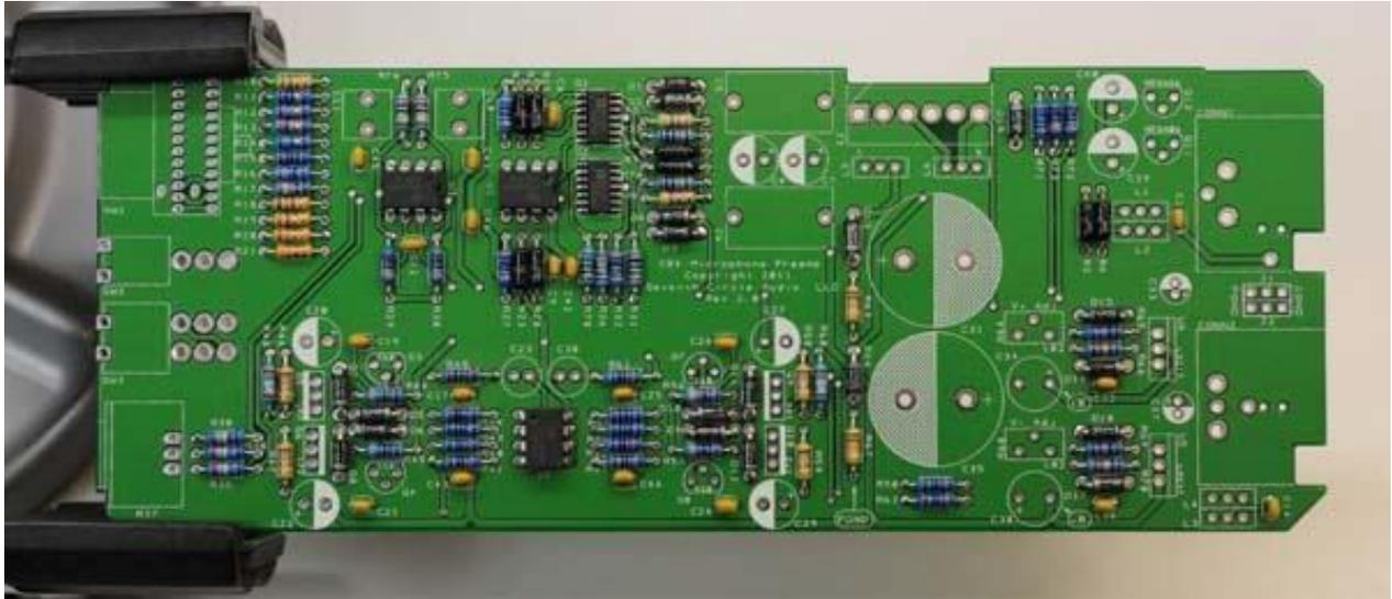
11. Install the ferrite filters now. These parts are not polarized and can be installed in either direction.
