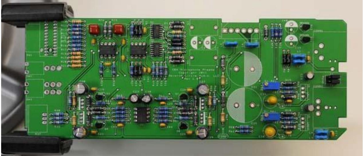
19. Add transistors Q5, Q6, Q9, and Q10. **Make sure to install the transistors correctly!** These parts are not the same and are not interchangeable. The heavy line on the silkscreen outline indicates the **back** of the transistor, the side **without** markings. **Make absolutely sure you don't insert them backwards.**
