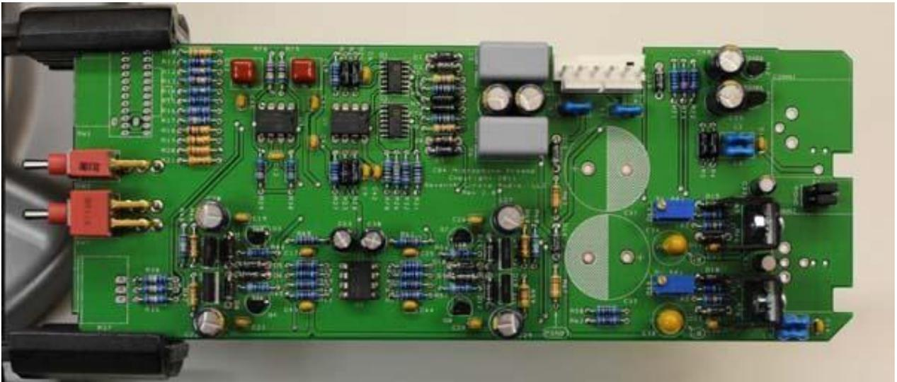
25. Install rotary switch, SW1. Make sure the switch is fully seated and solder it to the board. Try to make your solder joints as neat as possible, and don't use too much solder.
