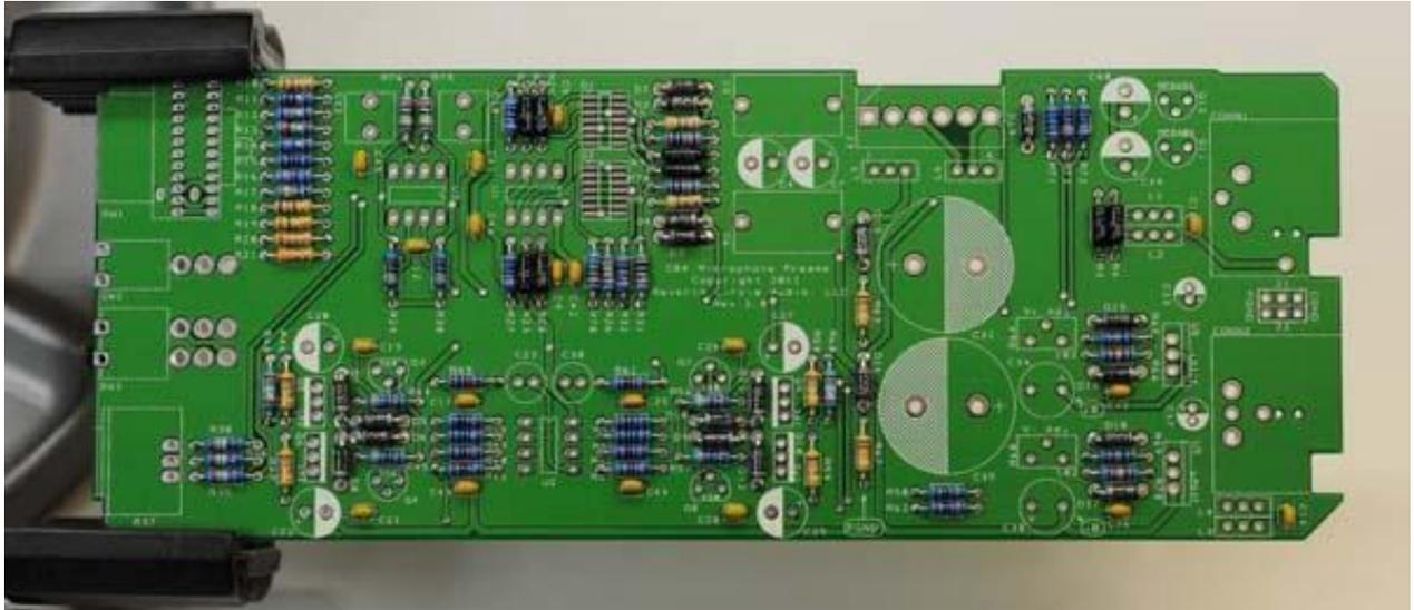
7. Install Q1 and Q2 now. Start by flowing a small amount of solder on two pads only as shown.
