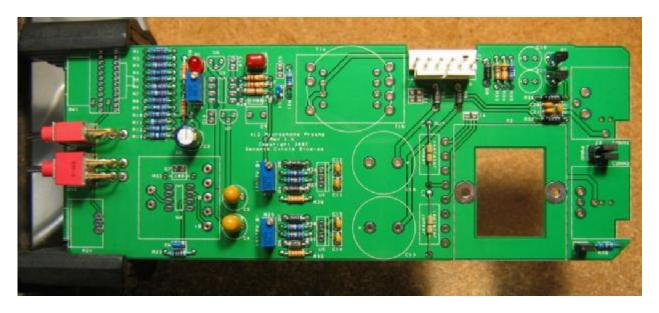
17. Install C16 and C17, the phantom power filter caps. Aluminum electrolytic capacitors are polarized and must be installed the right way round! Again, be absolutely sure to observe the correct polarity when installing these parts. The negative leads of the electrolytic caps are marked with a colored stripe. The positive pads on the circuit board are marked with a small "+" sign.
