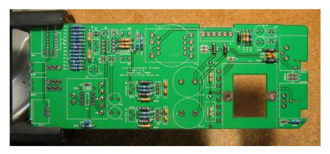
**8.** Add film capacitor C8. This capacitor is not polarized and can be installed in either direction.
