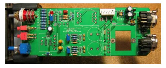
**24.** Attach the input transformer T1. **Don't forget to install the gray fish paper insulator under the transformer.** Pin 1 on the transformer is clearly indicated with a red dot.
