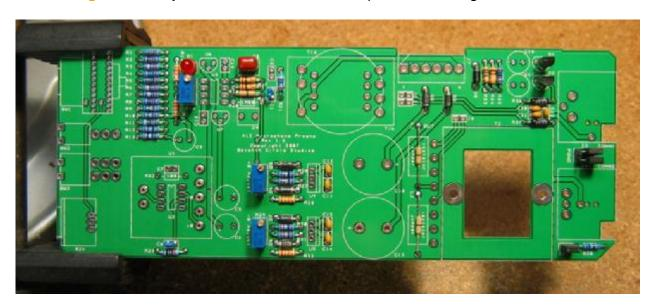
13. Add aluminum electrolytic capacitors C3, C12, and C15. Aluminum electrolytic capacitors are polarized and must be installed the right way round! Be absolutely sure to observe the correct polarity when installing this part. The negative lead of the capacitor is marked with a colored stripe. The positive pad on the circuit board is marked with a small "+" sign.
