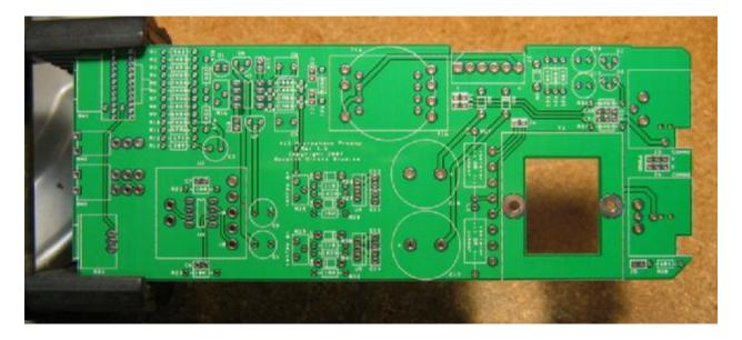
3. The first components to place are the Mill-Max receptacles. Press them into the holes using the point of a Philips screwdriver or similar tool. Be sure to support the board from behind while applying pressure. Push the sockets in firmly until they're flush with the board, and solder them from the back.
