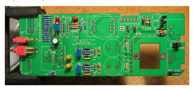
**16.** Add J7, the MOLEX power connector. Be sure to orient it as shown, with the locking tab away from the edge of the board.
