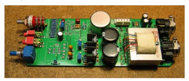
**29.** That's it! Before going on to initial power-up, carefully check your work. Make sure you haven't created any solder bridges between pads, or between a pad and the ground plane.
