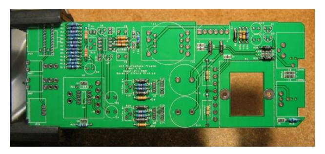
7. Add the ceramic capacitors C1, C6, C11, C14, and C20 – C22. These capacitors are not polarized and can be installed in either direction, but pay close attention to the capacitor markings! These parts all look alike, but they are not interchangeable. Putting one in the wrong spot will not prevent the preamp from passing signal, but it can seriously impair its performance. For the standard A12 with a discrete op-amp, don't install anything at C2, C7, C18, or C19.
