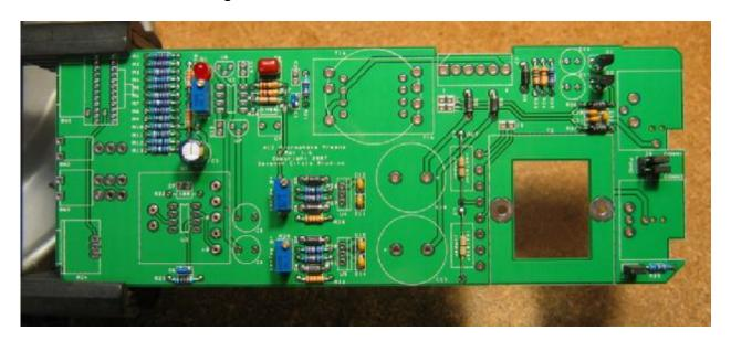
14. Add tantalum bypass capacitors C4 and C5. Tantalum electrolytic capacitors are polarized and must be installed the right way round! Be absolutely sure to observe the correct polarity when installing these parts. The positive leads of the tantalum caps are marked with a small "+" sign. The positive pads on the circuit board are marked with a small "+" sign.
