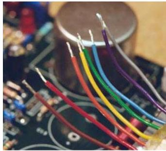
26. Solder the transformer leads to the circuit board as shown. The wire color is silk-screened next to each pad. The leads should not cross over and should be trimmed to the length shown. Do not leave the leads un-trimmed.
