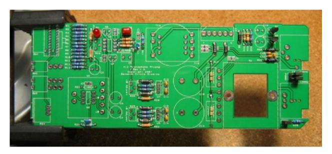
**12.** Install trim pots R16, R25, and R29. These parts are not the same and are not interchangeable! Pay close attention to the component markings.
