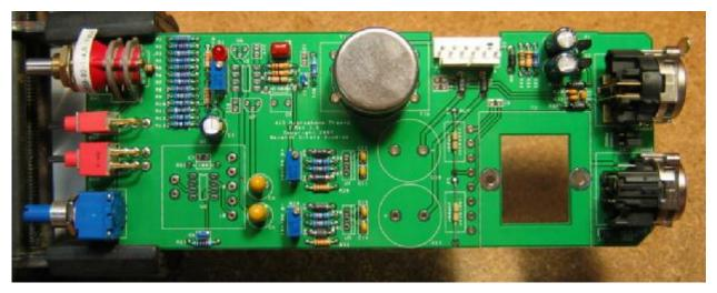
25. Using two #4-40 x 1" screws, attach the output transformer to the board. Place a 1/8" spacer on each screw between the transformer and the circuit board. Secure each screw with a #4 keps nut. Trim the leads to length, then strip and tin them with solder as shown. Tinning the leads makes them easier to manage in the next step.
