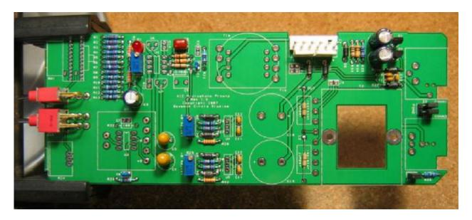
**18.** Attach gain trim control R24. Make sure the control is seated flat to the board before soldering the leads. You may want to add a small dab of silicone adhesive to the bottom of the control to hold it more securely.
