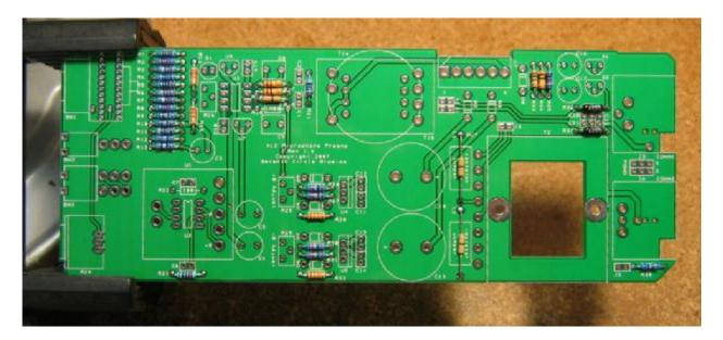
6. Next, add the protection diodes D2 – D8. Diodes are polarized and must be installed the right way round! The colored band on the diode matches the white band on the silkscreen.
