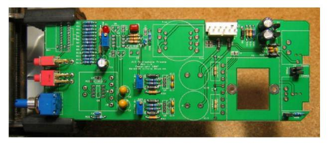
**19.** Insert the stop pin in rotary switch SW1 at the position shown. Push the pin in completely.
