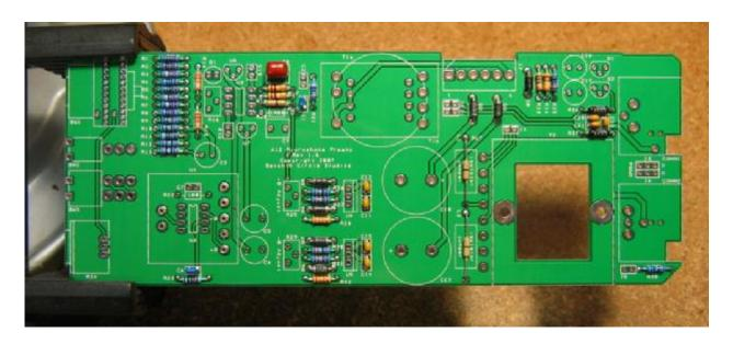
9. Add the 0.1" headers. You may find it easier to handle the headers if you attach the shorting jumpers before soldering. Install the headers with the long pins up! The function of the headers is as follows:
